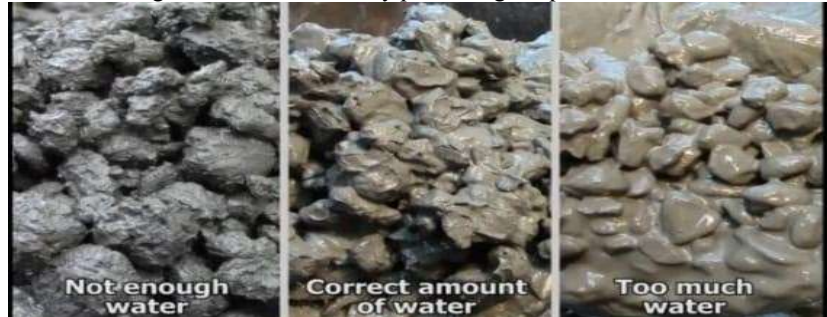
Fig. 10: Effect of Water Content on the Workability of Permeable Concrete
