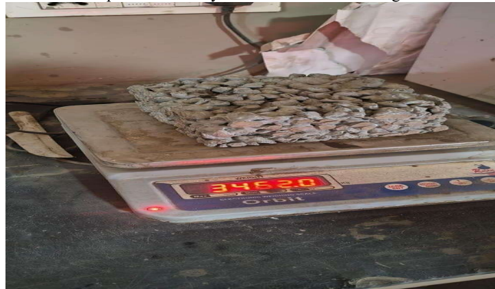
Fig. 11 Measurement of Weight of Permeable Concrete Specimen using Digital Weighing
