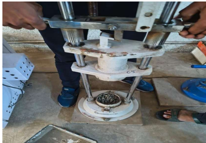
Fig. 14: Compaction of Aggregate Specimen using Compression Machine
