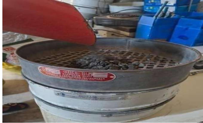
Fig. 13: Coarse Aggregate Placement for Sieve Analysis Test
