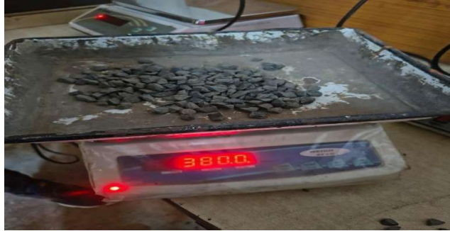
Fig. 15: Weighing of Coarse Aggregate using Electronic Weighing Balance
