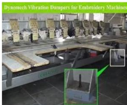
Figure 12. Vibration damping solutions for textile machines
