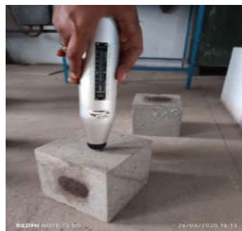
Fig.3 Rebound Hammer Test
