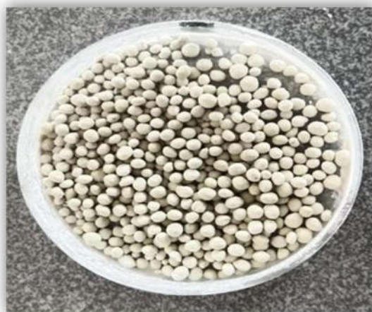
Fig 6.10 Soft Rupturable Beads By Using Extrusion- Spheronization [B4]
